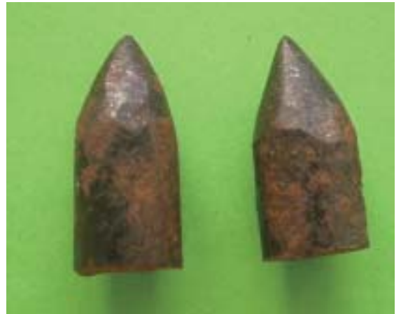
Figure 3. Forged bullets for a shotgun produced by cutting and sharpening 12-mm metal construction rods.
