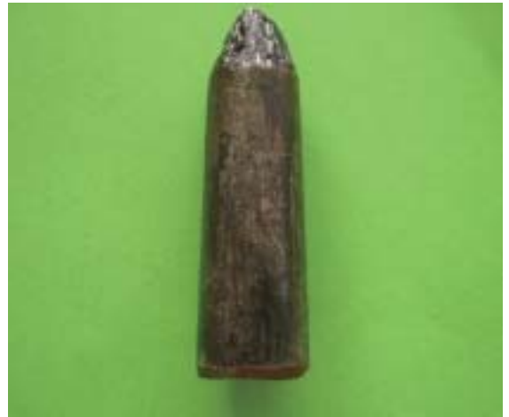
Figure 2. Slug for a shotgun produced by melting bullets or missiles of 12-mm cartridges and solidifying them in a 12-mm plastic cup.
