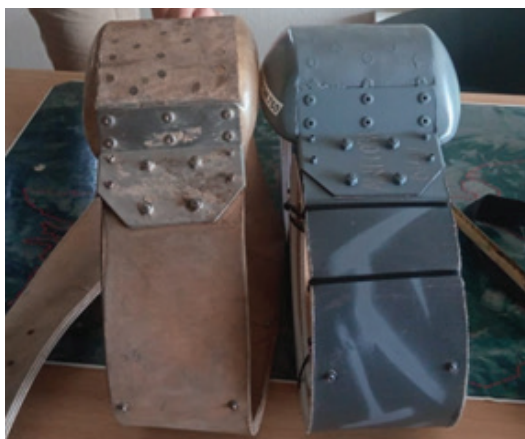
Figure 8. The original XL LoRa collar after it was removed from Kamva (left) and the refurbished LoRa collar that was fitted on Balu (right). (© Chris Reynecke)
