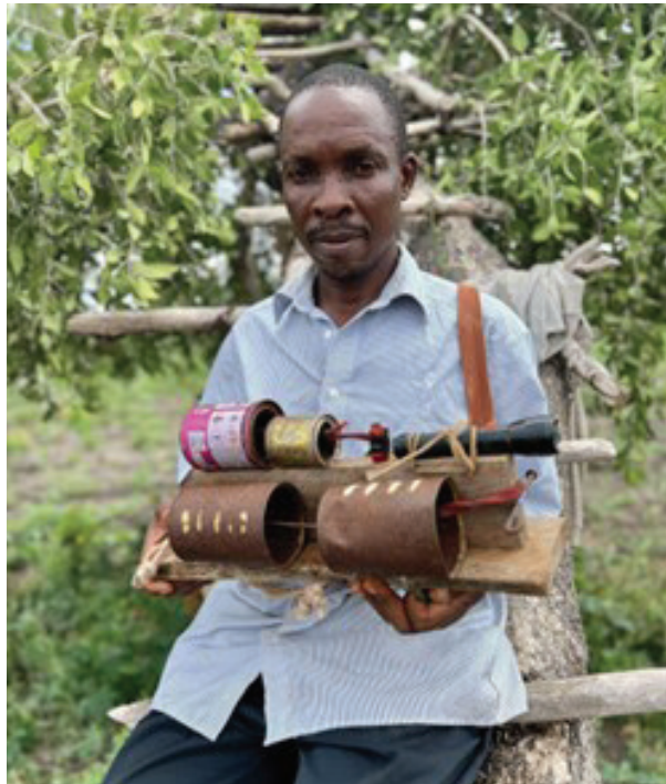
Figure 6. Living near Tsavo East NP in Kenya, Jones Mwakina, a farmer displays his homemade noise cannon device designed to scare elephants away from his farm. (© Jane Wynyard/Save the Elephants)
